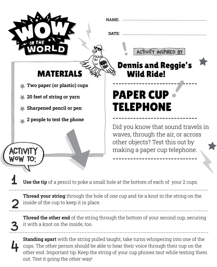
What in the WOW happened? Sound waves can travel through air, solids, and liquids. When you speak into the cup, the vibrations are transmitted into the string. They continue to travel through the string, as long as it is held taut, to the receiving cup. There the vibrations are transmitted to the air in the cup, around the listener's ear, allowing the whisper to be heard.
